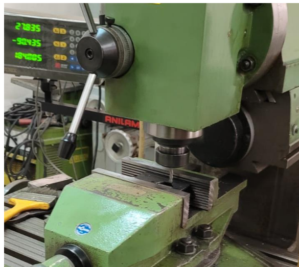
Figure 3: Milling process of the motor holder
